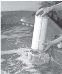
1) Center filter cartridge over canister
